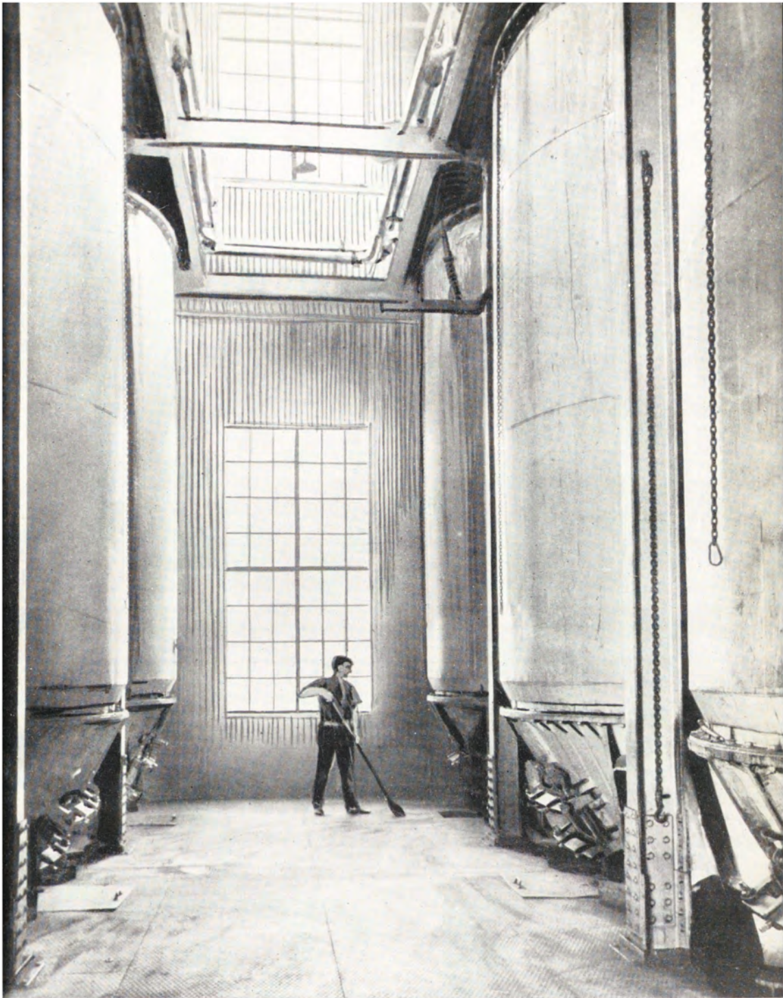
Char cisterns, Cottesloe Refinery ( from a retouched photograph ). Filtered "raw liquor" is run through cisterns containing granular bone char, which removes colouring matter and mineral constituents. The char is made by heating bones in closed retorts at high temperatures. It consists largely of calcium phosphate in the form of a porous "skeleton" coated with active carbon. A large surface area of carbon is thus available to adsorb colouring matter and mineral salts from sugar solutions. After use the char is washed, regenerated by heating—which decomposes adsorbed organic material—and used again.
