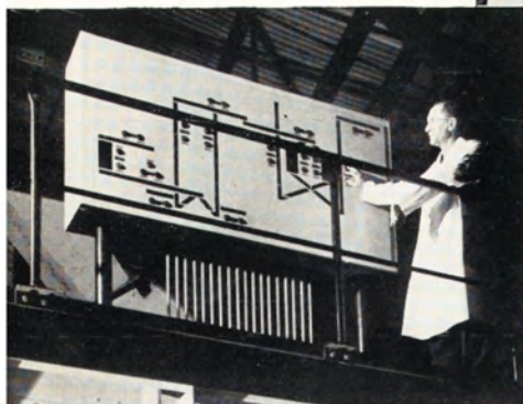
Control panel for belt conveyor system handling bulk raw sugar at Pymont refinery.
