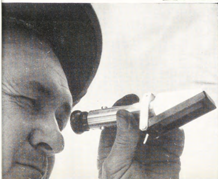
A drop of cane juice is poured on to the plate of a refractometer and the instrument is read. The refractometer measures the percentage of soluble solids in the cane juice, which gives a good indication of its sugar content.
