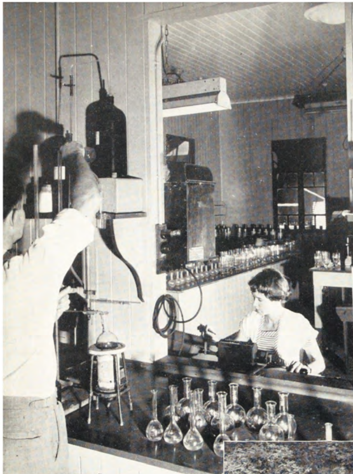
Laboratory, Victoria Mill. Chemists analyse the cane juice and syrups at various stages in the process, the megass, the molasses, the water in the mill mains, etc.
