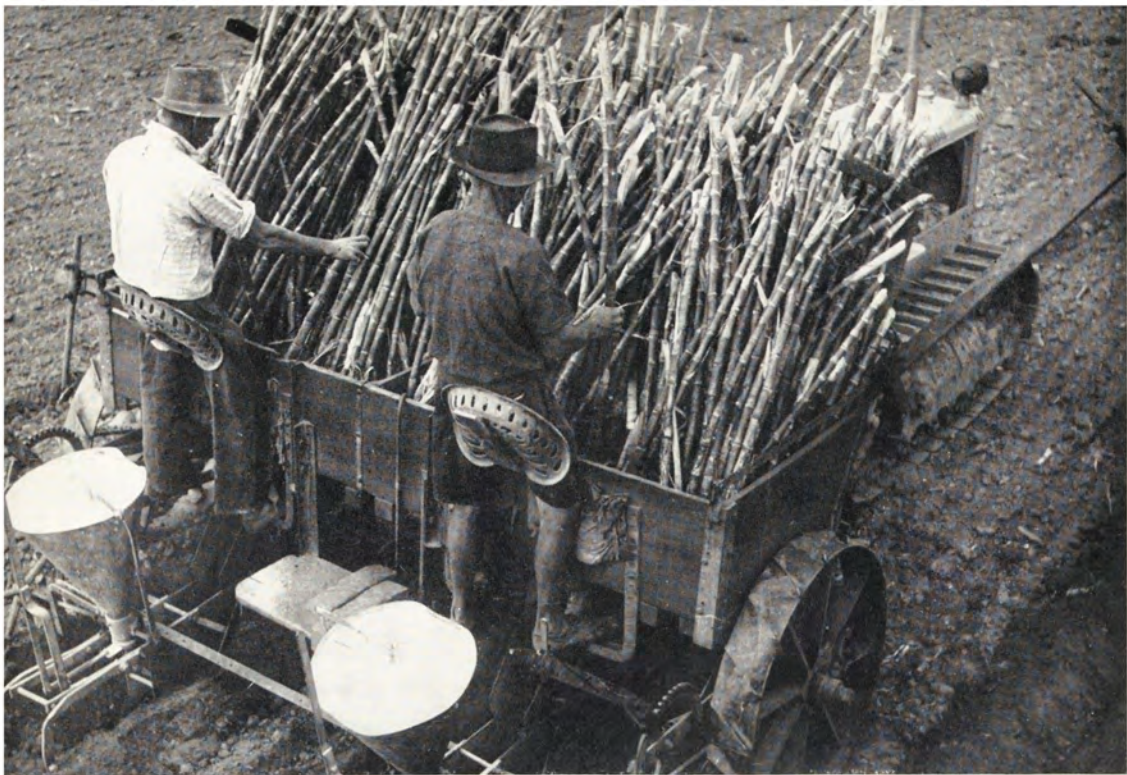
This double row planting machine cuts "seed" cane into one-foot lengths, drops the short pieces of cane into the furrows with fertilizer, and covers in the furrows as it moves along.
