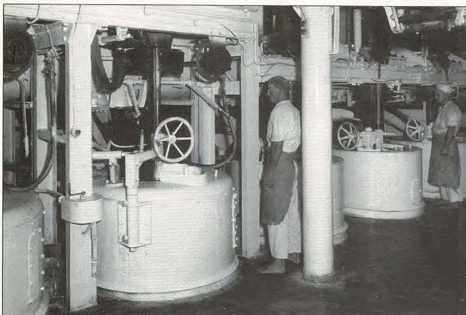
■ 48 inch and 42 inch refined centrifugals photographed in 1957. These manually operated refined fugals were replaced with an automatic system in the early 70s. Hessian bags were worn as aprons.
