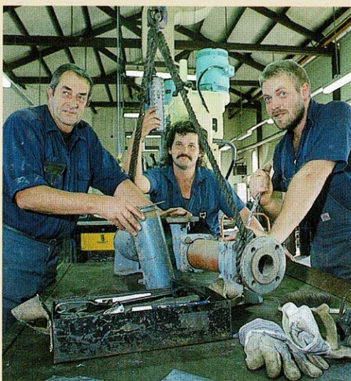
Foreman Graham Bright (left) checking a mono pump overhaul with trades assistant, Colin Webber, (centre) and fitter, Glen Bright.
