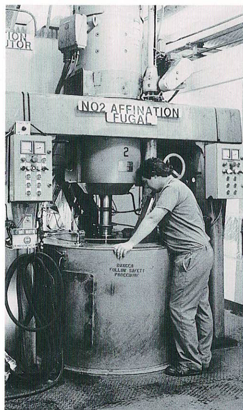
Steve Morrison keeps an eye on the fugalling operation shortly before the plant's closure.
