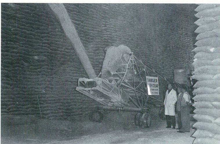
The "thrower" in action. Sugar conveyed to the raw store was thrown 100 feet in the air on to the raw sugar heap.
