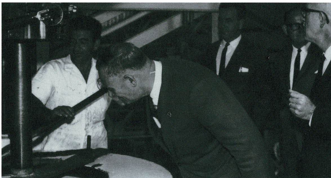
On a visit to the refinery in the mid 1960s, Sir David Brand (Premier of Western Australia, 1959-1971) peers into a fugal (centrifugal separator), operated by Tony Gurgone. Messrs. Vernon and McKenzie watch at right. Note that the fugal operator is using a paddle to plough out the sugar by hand.
